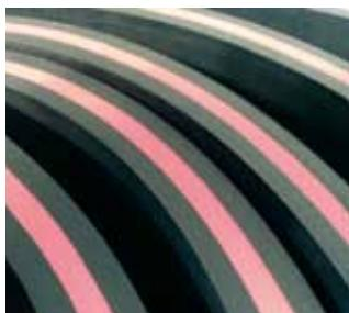
**USE:** RUBBER SCRAPER USED TO CLEAN THE BELT. IT IS COMPOSED OF THREE LAYERS OF RUBBER. THE TOP AND BOTTOM LAYER CONSIST OF HARDER BLACK, ANTI-ABRASIVE RUBBER, WHILE THE CENTRAL LAYER CONSISTS OF SOFTER, RED PARA RUBBER. THIS PARTICULAR STRUCTURE ENSURES THE PRODUCT IS VERY LONG-LASTING AND GIVES EVEN CLEANING. - **SURFACE:** SMOOTH/SMOOTH
